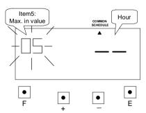
Press the [+] or [-] button to set at "05" and press [E] button. At the same time, the flashing changes from "Item5" to "Hour".
