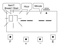
Press the [+] or [-] button to set at "07" and press [E] button. At the same time, the flashing changes from "Item6" to "Hour".
