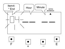
Press the [+] or [-] button to set at "04" and press [E] button. At the same time, the flashing changes from "Item4" to "Hour".
