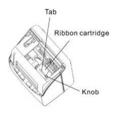
(3) Turn the knob of the new cartridge in direction of the arrow (clockwise) to tighten the ribbon.
