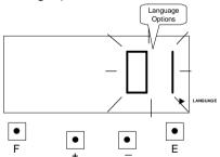
(2) Such as example, press the [+] or [-] button to set at "2", and then press [E] button. At the same time, the LCD screen only display "▲" under the "DATE IMPRINT" mark.
