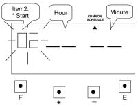
Press the [+] or [-] button to set at "02" and press [E] button. At the same time, the flashing changes from "Item2" to "Hour".
