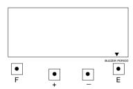
(4) If you want to set another function, press the [F] button to continue setting. If you finished setting the functions, replace the cover and lock it.
