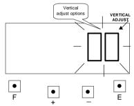
Such as example, Press the [+] or [-] button to set at "2", and then press the [E] button.
