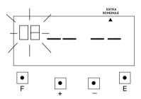
h. Setting the Item8 (Break1 End) **Example:** break1 end time is set at 10:15.
