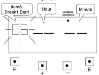
Press the [+] or [-] button to set at "06" and press [E] button. At the same time, the flashing changes from "Item6" to "Hour".
