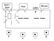
Such as example, press the [E] button because the item is not to be changed. At the same time, the flashing changes from "Item1" to "Hour".
