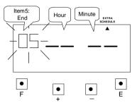
Press the [+] or [-] button to set at "05" and press [E] button. At the same time, the flashing changes from "Item5" to "Hour".
